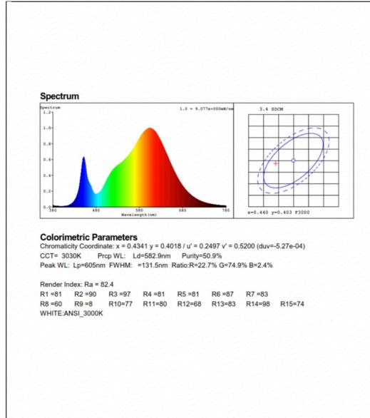
Attachment 1: Photometric test record of one lamp at initial measurement
